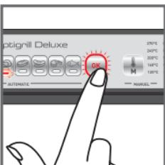
11 Press the « SELECT » button several times until you reach the desired program. **Ensure that there is no food inside the grill.** When you have selected the wishing one then press the « OK » button.
